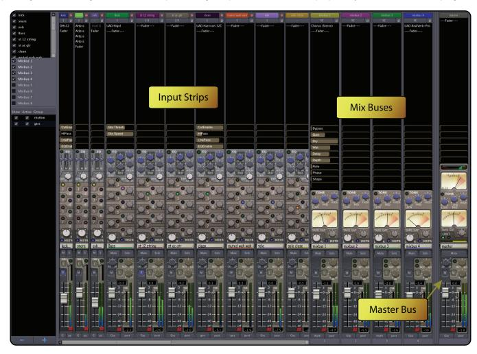
In Mixbus, like other audio workstations, each recording track has its own mixer strip. These mixer strips resemble the input channels of a traditional analog mixing console. Input channels can be configured to be mono or stereo and by default include all the DSP processing that makes up a real console channel. This is the major difference between Mixbus and other DAW mixers. No time is wasted searching for and adding the necessary high-quality mixing tools.
